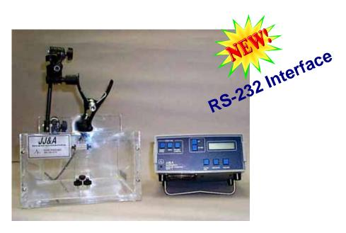
The Mark 4 *Plus* Doppler phantom is a very accurate device for testing Doppler ultrasound scanners. It is especially useful for checking sample volume registration, color registration, directional discrimination, and Doppler velocity accuracy.
