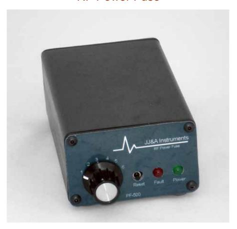
The PF-500 is a stand-alone RF power sentry that is used to protect expensive transducers from accidental overpower damage. Placed in-line between the RF power generator and the transducer, it passes the signal unless the power level exceeds the desired limits. The user may select from six power-limit settings. If an excessive amount of power is sent to the transducer, the PF-500 will send out a warning signal or short the RF line to ground, or both, depending on the user settings.
