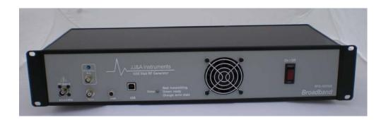
The RFG-1500BB provides the HIFU researcher with a powerful tool to replace stacks of laboratory equipment such as signal generators, pulse generators, timing circuits, and power amplifiers.
